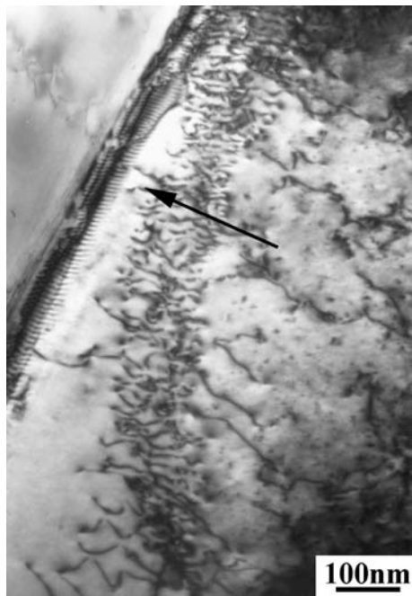
Fig. 8 TEM bright field image of a MB2's wall formed following 50% strain at 650 °C (arrowed). The dislocations form arrays of parallel dislocations
